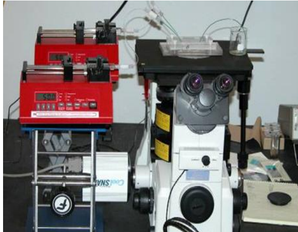
Figure 2. Photograph of the experimental set-up showing the microscope, syringe pumps and the microfluidic device fitted in the interconnect.
