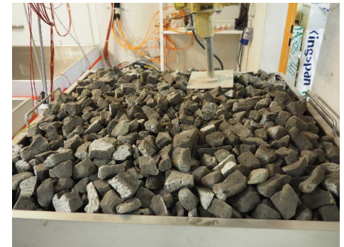
Compacted FFG (30 %) Compaction process
