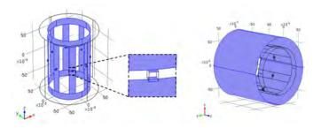
FEM Models of Birdcage Coils Frequency Domain Analysis Eigenfrequency Analysis Software Tool
