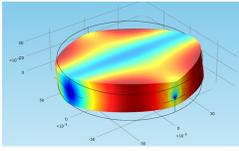
**Figure 1:** Eigenfrequency response of at cut quartz crystal upon loading
