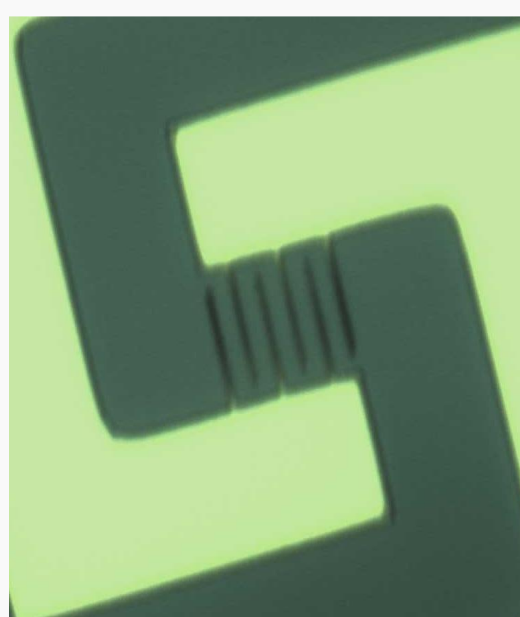
Photograph of a 9x9 μm physical photomixer: "finger" electrodes visible in center of image.
