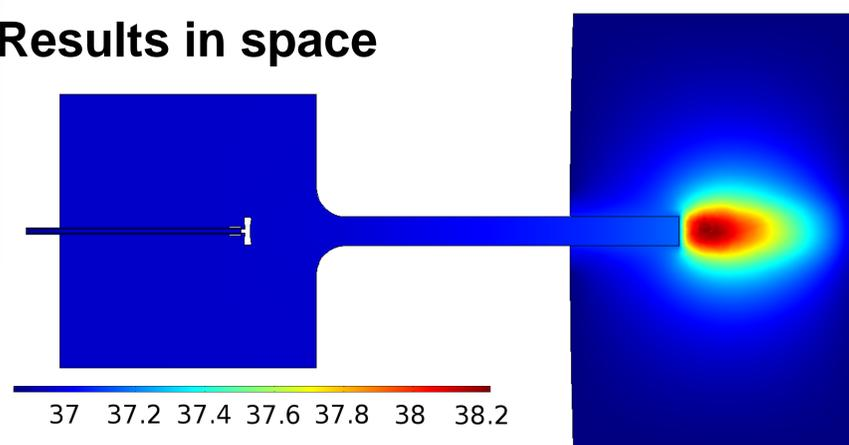
Figure 6. Temperature distribution (°C). The results show us that we can reach 1-2°C temperature rise within 4mm radius area at the tip of the device in case of 10mW laser power. The silicon shaft remains cold due to the low absorbent coefficient for infrared light and the high heat transfer coefficient compared to brain material.
