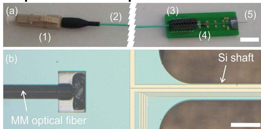
Figure 2. Perspective view of packaged INS microelectrode (a) (1) LC optical connector, (2) Multimode optical fiber, (3) PreciDip electrical connector, (4) Printed circuit board, (5) microchip. Close view of coupled fiber
