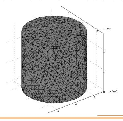
Geometry of the LDA interaction focusing volume for  $\lambda = 1.06~\mu m$  incident wavelength. The COMSOL mesh grid can be observed.
