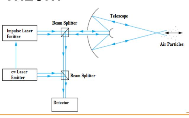
Example of LDA setup schematic.
