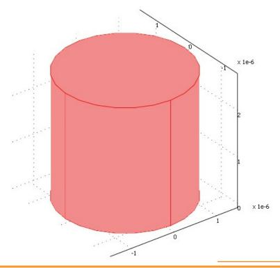
Geometry of the LDA interaction focusing volume for  $\lambda$  = 1.06  $\mu$ m incident wavelength.
