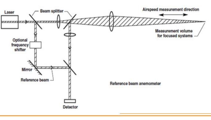
Example of LDA setup schematic.
