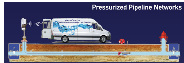
Figure 16. Electro Scan Inc. set-up in pressurized water mains.
