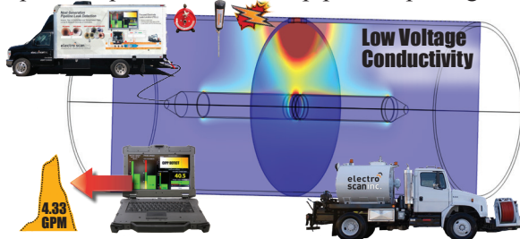
Figure 11. Use of COMSOL to confirm quantification of defect electric current of low voltage conductivity.
