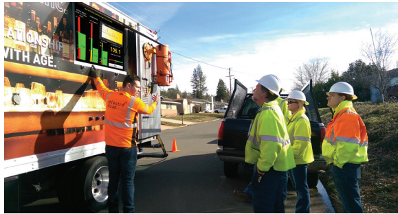
Figure 18. Electro Scan showing real-time defect identification in the field.
