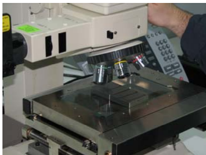
Figure 5. Measuring the depth and width of engraving on the block of Steel 1.2767
