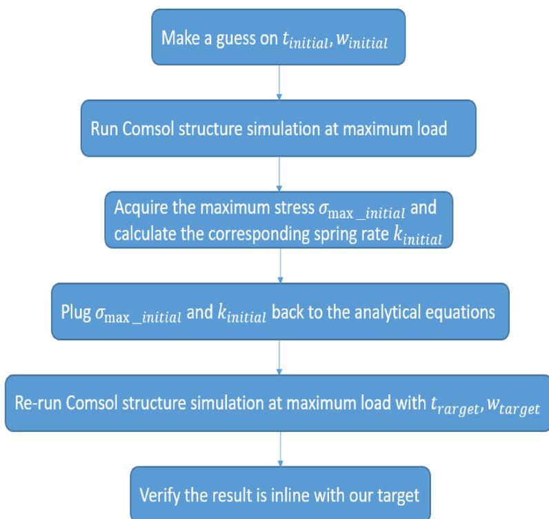
**Figure 1.** The flowchart of non-coiled spring optimization of utilizing FEM model assisted by an analytical model
