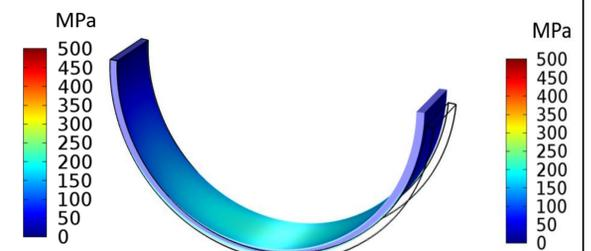
**Figure 3.** Stress distribution of the spring with assisted analytical model predicted design variable value:
