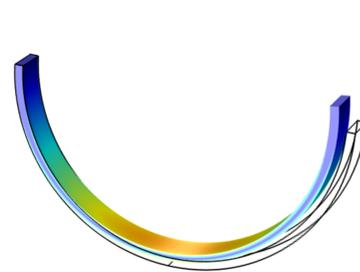
**Figure 2.** Stress distribution of the spring with initial guessed design variable value:
