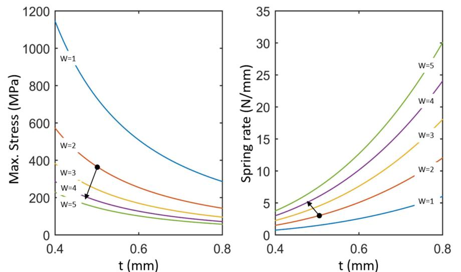
**Figure 4.** Spring performance w.r.t. design variable space. The arrow represents the optimization trajectory.
