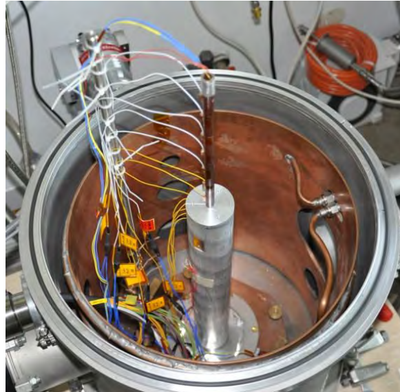
Unshielded configuration ( surface-to ambient radiation)
