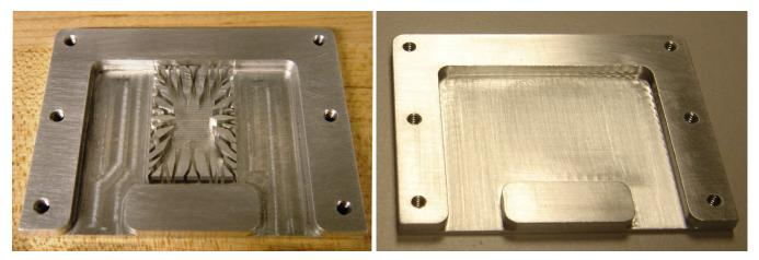
Prototype aluminum cold plates with (left) and without (right) a representative hierarchical microchannel topology.
