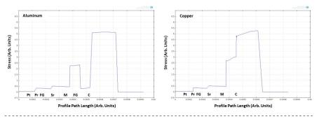
Relative stress in arbitrary units was plotted through the depth of the composite structure layups containing either aluminum (left) or copper EMF (right).
