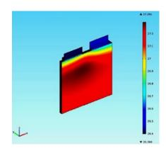
Surface temperature of a pouch cell from a lithium ion battery pack - the uniform distribution is an important parameter
