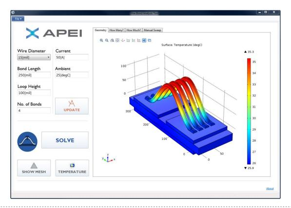
The application showing the temperature change in the wire bonds. The end user chooses the bond length, loop height, current level, and number of bonds.
