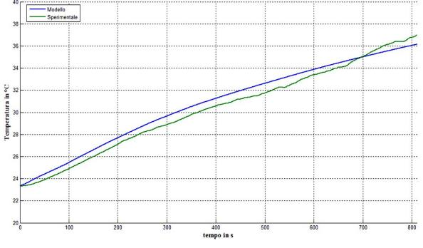
A comparison of model and experimental results for one of the thermocouples on the surface of the lithium cell. The results show a maximum difference of 1°C between the two.
