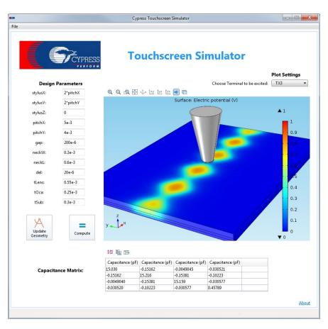
Simulation app based on a COMSOL® software model used to support the design of touch-based capacitive sensors. The app user can change design parameters ranging from the finger location to the thickness of different layers in the sensor. A drop-down list can be used to select a solution corresponding to the excitation of different sensor traces.
