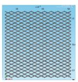
At left is the composite structure layup from the COMSOL Multiphysics" software model and, at right, the geometry of the expanded metal foil. SWD and LWD correspond to short way dimension and long way dimension. The mesh aspect ratio, SWD/LWD, is one of the parameters varied in the study.
