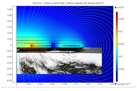
Comparison between results from COMSOL Multiphysics<sup>\*</sup> software (magnetic flux density norm) and experimental field lines can be used to test other coil designs before building a prototype.
