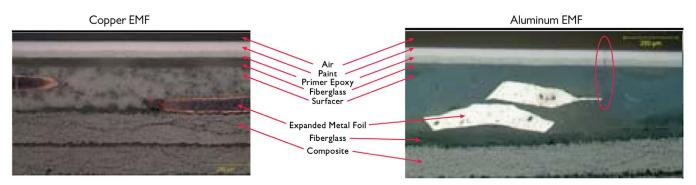
Photo micrographs of the composite structure layups after exposure to moisture and thermal cycling. At left, the results for the copper EMF and at right, the aluminum.
