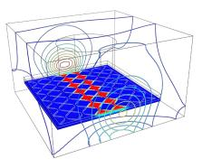
Example design box showing a touch sensor with electric field lines modeled using the AC/DC Module, an add-on product to COMSOL Multiphysics<sup>\*</sup> software.
