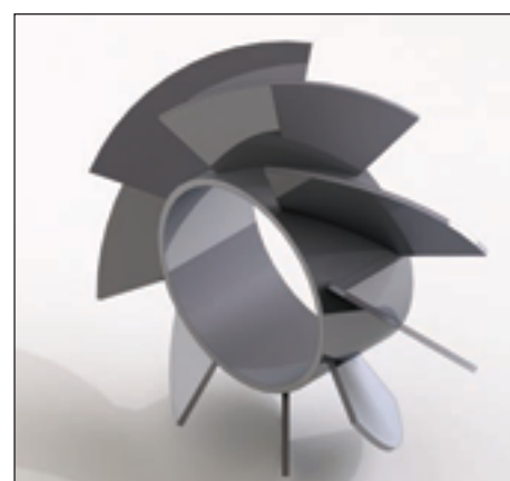
Figure 2: Geometry of the axial swirler.
