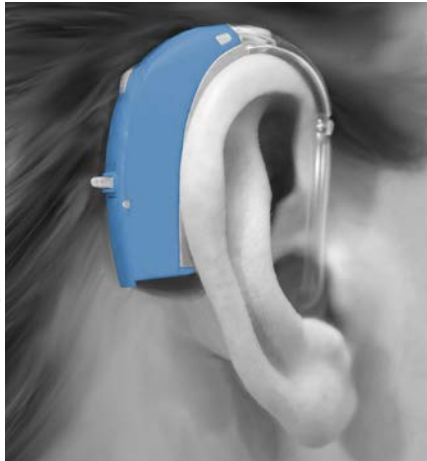
FIGURE 1 A typical BTE hearing aid includes microphones, vibration insulation, and a receiver, among other components. The tight spacing of these components invites troublesome acoustic and mechanical feedback. (Image credit: Knowles Corp.)
