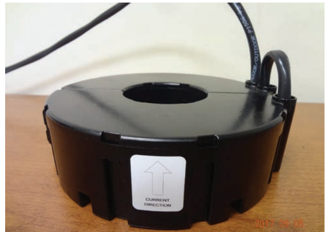
Figure 6. The submersible split-core sensor.
