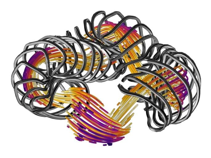
Figure 1: Non-planar HTS coil system of a stellarator fusion reactor modeled using the homogenized T-A formulation.
