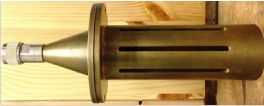
Figure 1 : Geometry of the coaxial cell for dielectric measurement and microwave heating applicator
