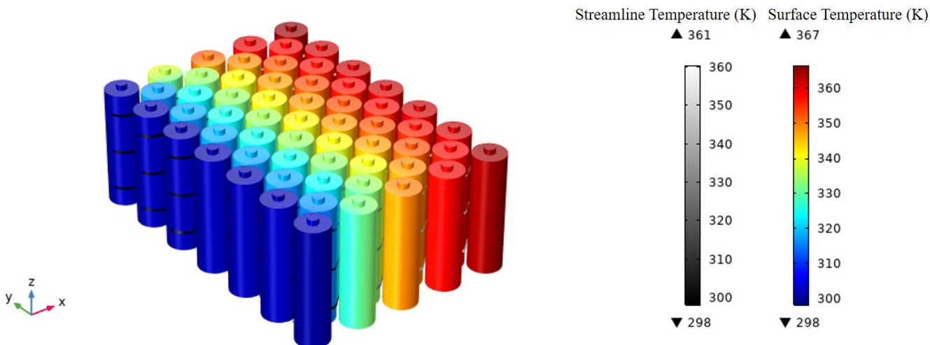
Figure 2 : Temperature Profile for a Battery Module with 59 Cells
