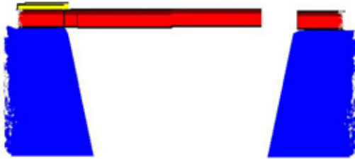
Figure 3: A cross-section of a fixed-free type cantilever device (dimensions are not to scale). The n^{++} silicon is dark red, the n^+ layer is red, the middle oxide is black, the substrate is blue, and the gold pad-metal is yellow.
