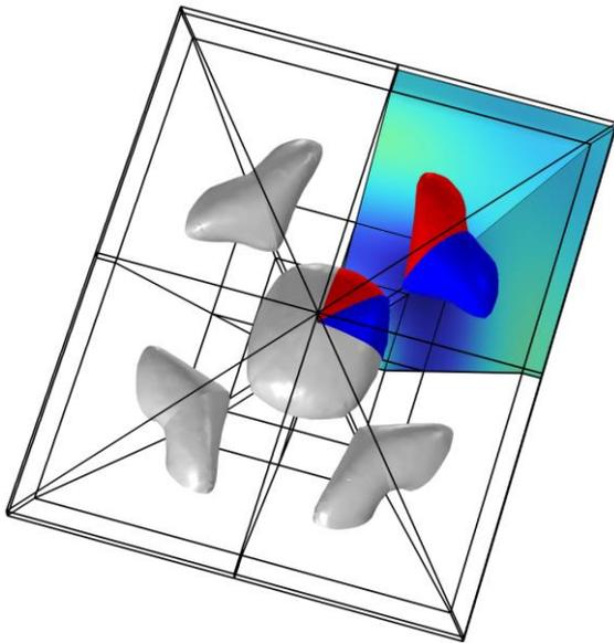
Figure 4: A rectangular waveguide with quarter symmetry and a scale-mirror-scale constrained acoustic lens. The blue parts are the design variables mapping to the red parts, with the grey parts completing the lens.
