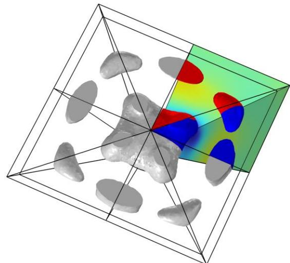
Figure 3: A square waveguide with quarter symmetry and a mirror constrained acoustic lens. The blue parts are the design variables that map to the red parts, with the grey parts completing the lens.
