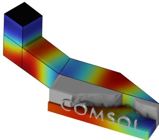
Figure 10: The black boundary has an acceleration input with the gray domains showing the topology optimized design.
