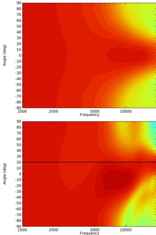
Figure 2: Initial tweeter vertical plane directivity (top) and optimized ditto (bottom) with a line at 20 degrees.
