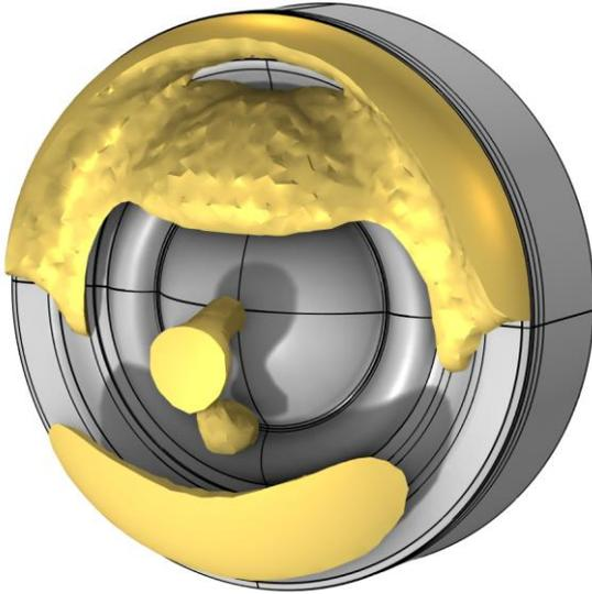
Figure 1: A tweeter has been fitted with a topology optimized lens.
