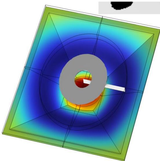
Figure 7: Elliptical rotation constrained lens for a rectangular waveguide, with the 2D optimized section.
