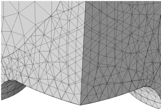
Figure 9: Incompatible and overlapping meshes because of field/mesh export of optimized design and subsequent import into the initial geometry.
