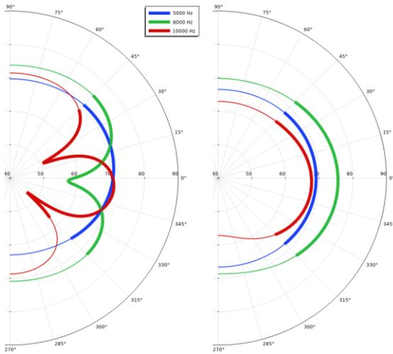
Figure 11: The horizontal radiation pattern before (left) and after optimization (right) for three frequencies with the focus being on  $\pm 45$  degrees (bold lines).
