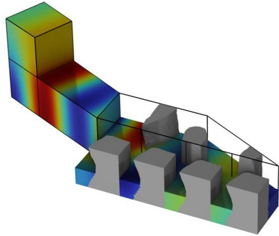
Figure 5: A repeating pattern has been obtained at the output of an acoustic conduit for the topology optimized structure (grey).
