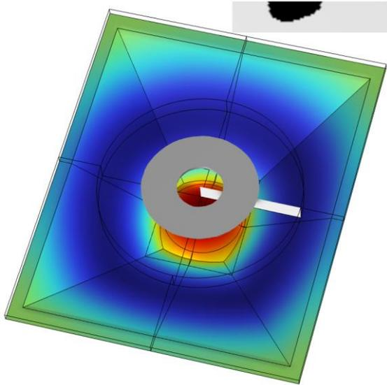
Figure 6: Circular rotation constrained lens for a rectangular waveguide, with the 2D optimized section.
