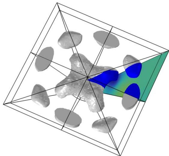
Figure 8: A square waveguide using 1/8<sup>th</sup> of a full 3D geometry with an equation-based mirror constrained acoustic lens. The blue parts are the design variables, with the grey parts completing the lens.
