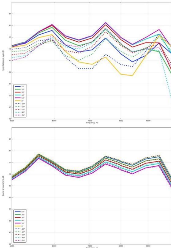
Figure 12: Sound pressure levels at certain horizontal angles before (top) and after (bottom) optimization.
