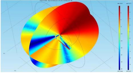
**Figure 4:** Skin thickness of 3100  $\mu\text{m}$  and fat tissue of 1.1 cm stretched across the antenna. Attenuation ranges from -3.9 to -8.5 norm dB.
