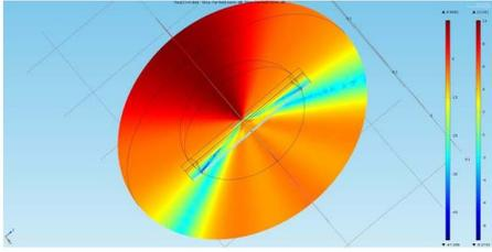
**Figure 2:** Skin thickness of 2600  $\mu\text{m}$  and fat tissue of 1 cm stretched across the antenna. Attenuation ranges from -3.1 to -7.3 dB.
