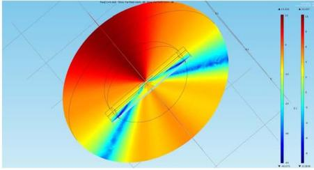
**Figure 3:** Skin thickness of 2900  $\mu\text{m}$  and fat tissue of 1.1 cm stretched across the antenna. Attenuation ranges from -3.4 to -8 dB.
