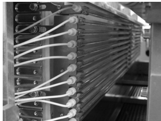
Figure 1. Photo of one IR lamp panel with preforms placed in front of it [SMI Group S.p.a.].
