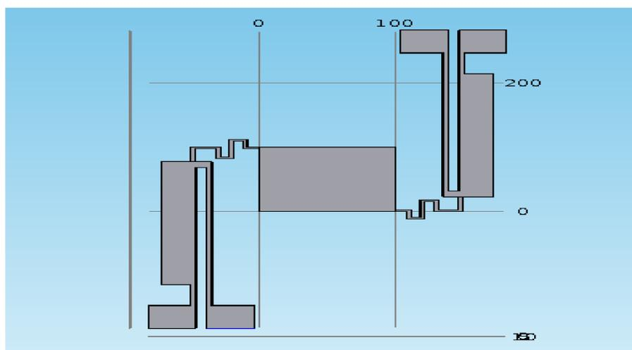
Figure 1. Structure of Micro-mirror with ETA
