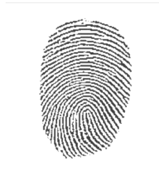
Figure 9b: The fingerprint image generated by rectangular microsensor
