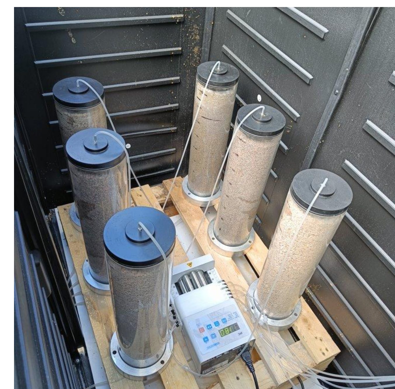
Figure 2: Column experiment realized in the summer of 2023 to test efficiency of Kymisand, Rådasand and Polonite in P and Fe retention.
