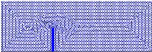
**Figure 2:** FSI Model of interaction of cardiomyocytes with a Microcantilever at  $t=0s$
