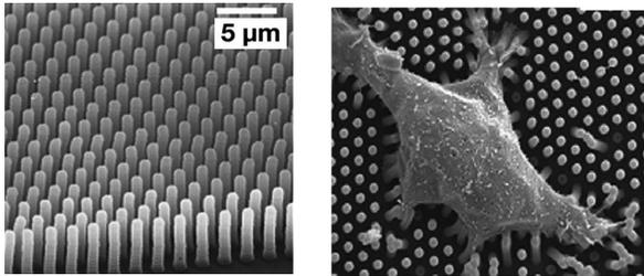
Scanning electron micrograph of closely spaced array of vertical microcantilevers produced using reactive ion etching techniques, and Individual MDCK cells attached to the array (From du Roure et al. (62), PNAS 102, 2390–2395, 2005, National Academy of Sciences, U.S.A.)
