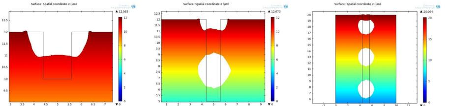
**Figure 2.** Number of final voids depending on the trench length/diameter ratio for values of (left to right) 1.67, 5.83 and 12.5
