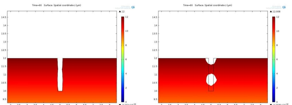
**Figure 3.** Evolution after 80 seconds annealing at a temperature of (left to right) 900 °C and 1100 °C
