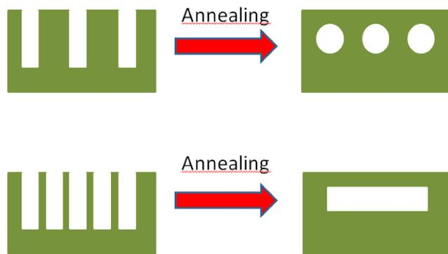
**Figure 1.** Void shape evolution scheme depending on the trench separation
