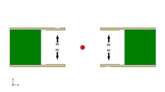
**Figure 1**: Cross section of one electrode segment in the xy-plane of the ion trap. Green domains are silicon substrate, grey domains are insulator, and orange domains are gold electrodes. The black arrows indicate where the AC and DC potential are applied and the red circle shows where the ion is confined.
