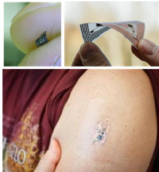
Figure 1. Ultra-thin chip bent between fingers (top left), Flexible monitoring tag (top right) 3 and skin temperature sensor patch (bottom).
