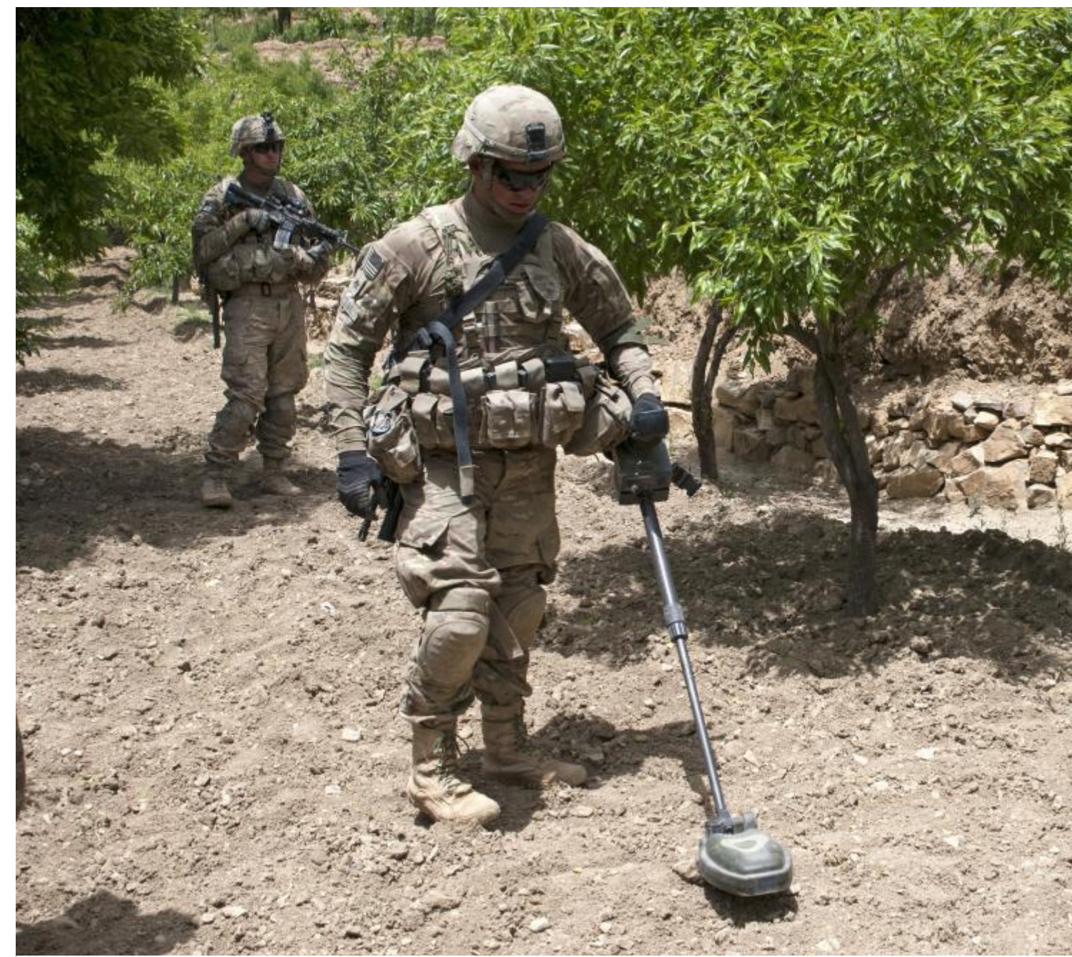
Figure 1: Pfc. Nikko Williams using an advanced EMI sensor called the VMR2 Minehound [2].
