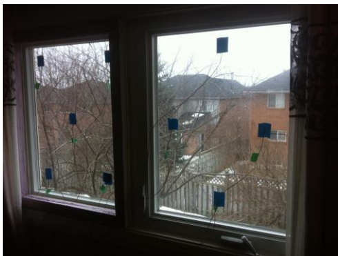
Figure 2. Windows, part of the OI system, and taped thermocouples used in the experiment in a test-home
