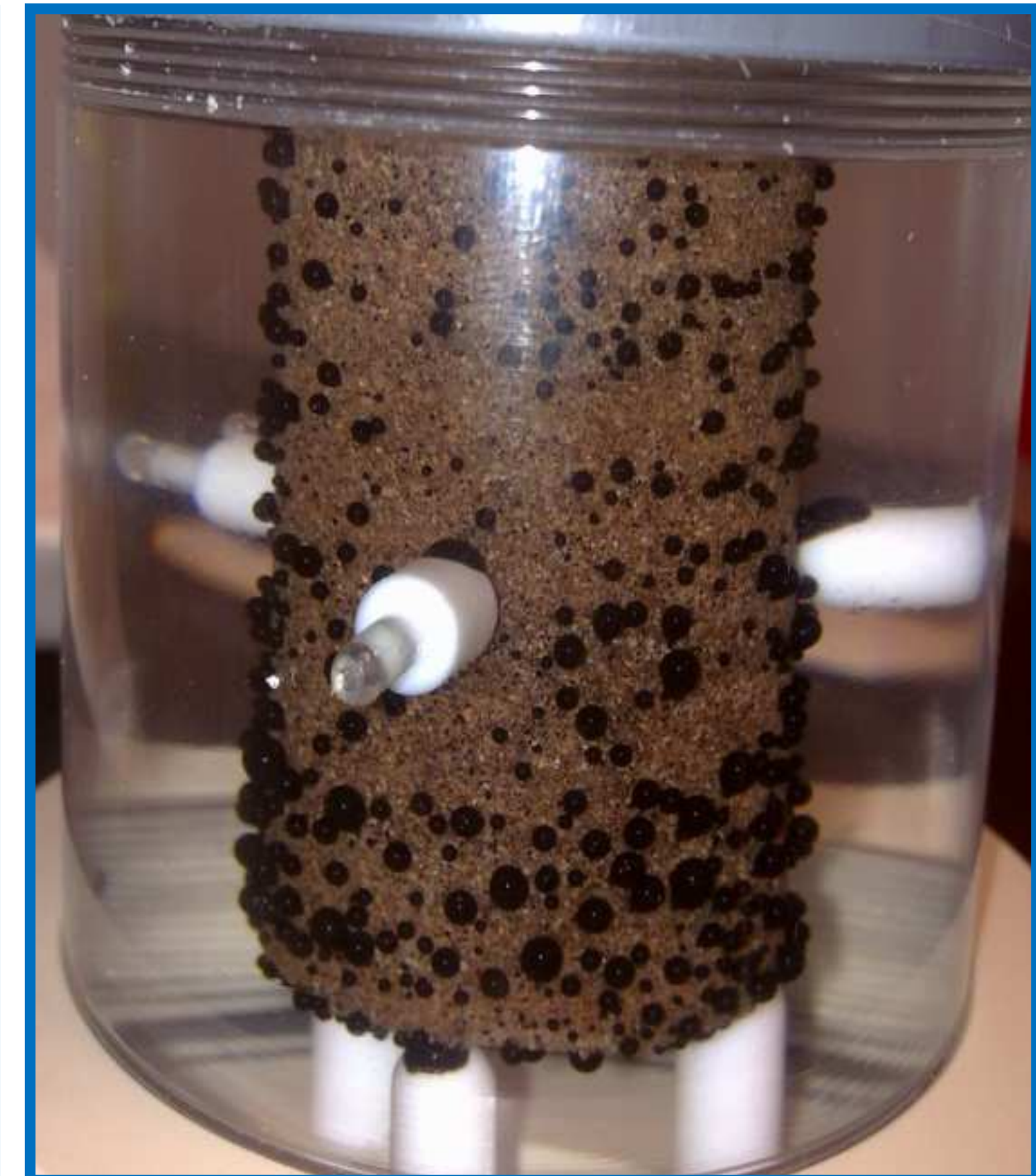
Figure 1. The process of penetration (Countercurrent imbibition) of MSS into an oil-filled core sample. Oil is produced from all boundaries.
