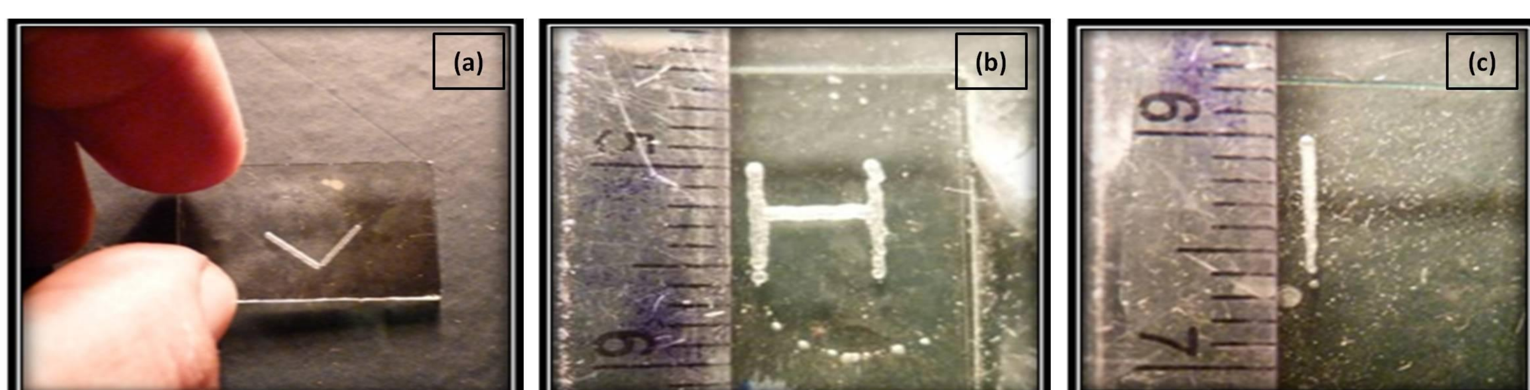
Figure 2. : Different types of Microchannels on Glass
