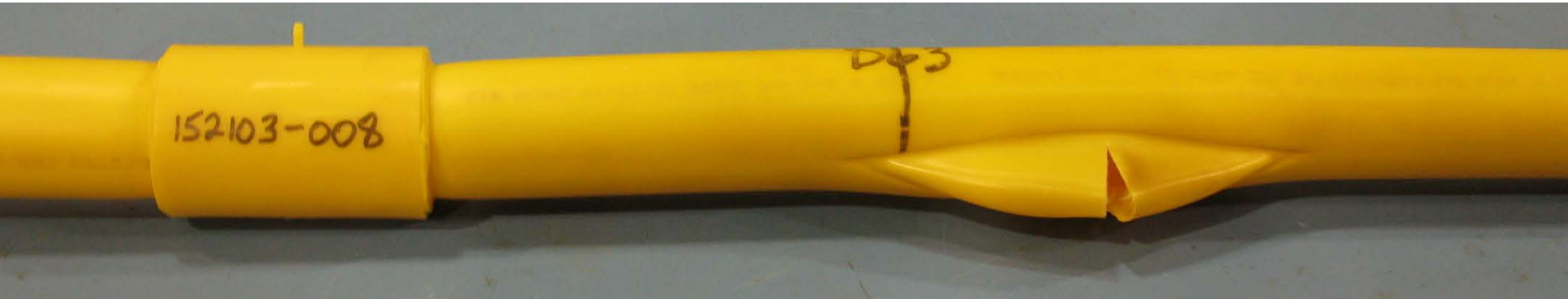
Classic ductile rupture
