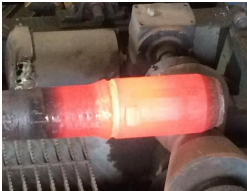
Pipe end preheating
