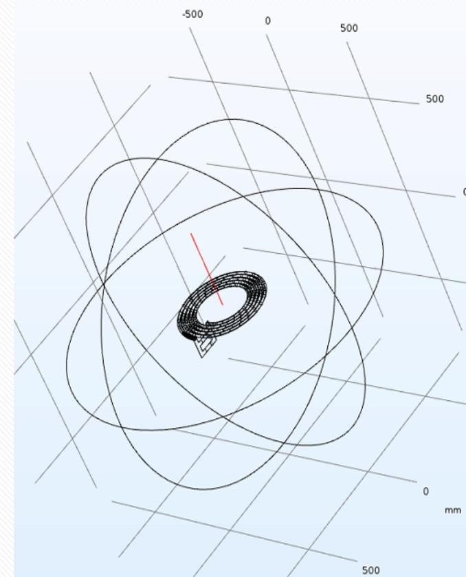
As the major radius and radial pitch combinations approach the dimensions of the coil measured at the lab, the magnetic field decay behaves similarly
