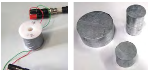
Figure 1. The air-core transformer (left) and the different shields
