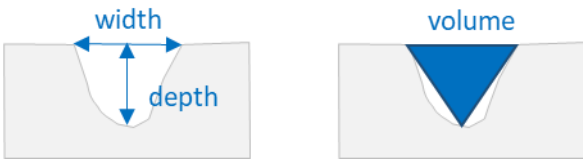
Figure 3. Graphical definition of ablated craters width, depth and volume.
